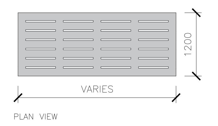
LENGTHS AVAILABLE IN 100MM INCREMENTS FROM 1800MM TO 3800MM PLUS 3950MM, 4100MM & 4250MM.
